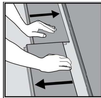
Fig 12 Disassemble the panels on the short side by sliding apart horizontally. NB Do not lift the short sides up.
