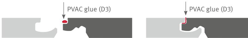
In industrial areas you have to anticipate extraordinary exposure to moisture. As a result, additional sealing with PVAC glue (D3) is mandatory for such applications. Apply the sealing glue to the top of the tongue on the short and long edge. The glue should ooze out along the complete long and short edge after the panels have been connected together. Excess sealing glue is easy to remove from the surface immediately or after a short drying period.
