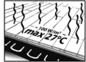
**NOTE ! A room ambient temperature on average can be approximately 5 degrees lower than the temperature of LVT flooring at floor level. Please consider this if setting ambient room temperatures rather than floor surface temperatures to ensure the flooring itself is not heated above 27 deg C.**
